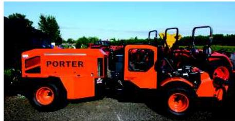
Porter Orchard Boss 125D tractor w/ 125HP Perkins tier 3 engine, front and rear three point and PTO, tight turning radius, low 5'6" height, 40GPM hydraulic outlets, hydrostatic transmission with 10 programmable set speeds, 4wd, and much, much more. **Sale Price: \$96,900**
