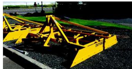
Domries 9' orchard leveler model OBL-9 SN. M13702 w/adjustable blades, 1/2" x 6" reversible blades, available in 8' to 18' widths, and 4 stage leveling. **ONE ONLY at \$3,500**
