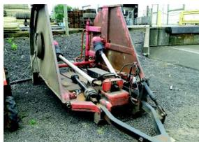
Bush Hog model 1625R wing-fold, 14' rotary cutter with single blades. Stock # 43382
